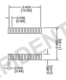
RECOMMENDED SOLDER PAD DIMENSIONS DIMENSIONS: Inch [mm]
