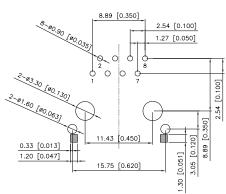
RECOMMENDED PCB LAYOUT (TOP VIEW)
