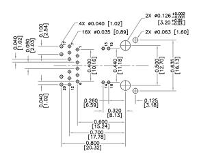
Recommended PCB Layout (Component Side)
