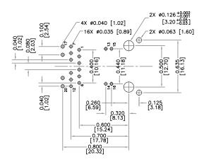
Recommended PCB Layout (Component Side)
