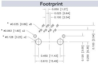
Recommended PC Board Pattern (Comp. Side) \*Adjust Hole Size Based on Customer Process Tolerances
