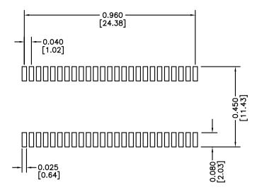
RECOMMENDED SOLDER PAD DIMENSIONS DIMENSIONS: Inch [mm]
