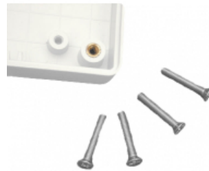
Standard models use machine screws into brass bushings. Economy models use self tapping screws.
