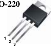
1.Gate 2. Drain 3. Source
