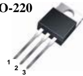
1.Gate 2. Drain 3. Source
