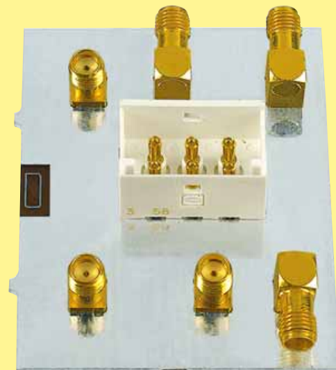
Fig. 6: Test boards with implemented Mini Coax connector
