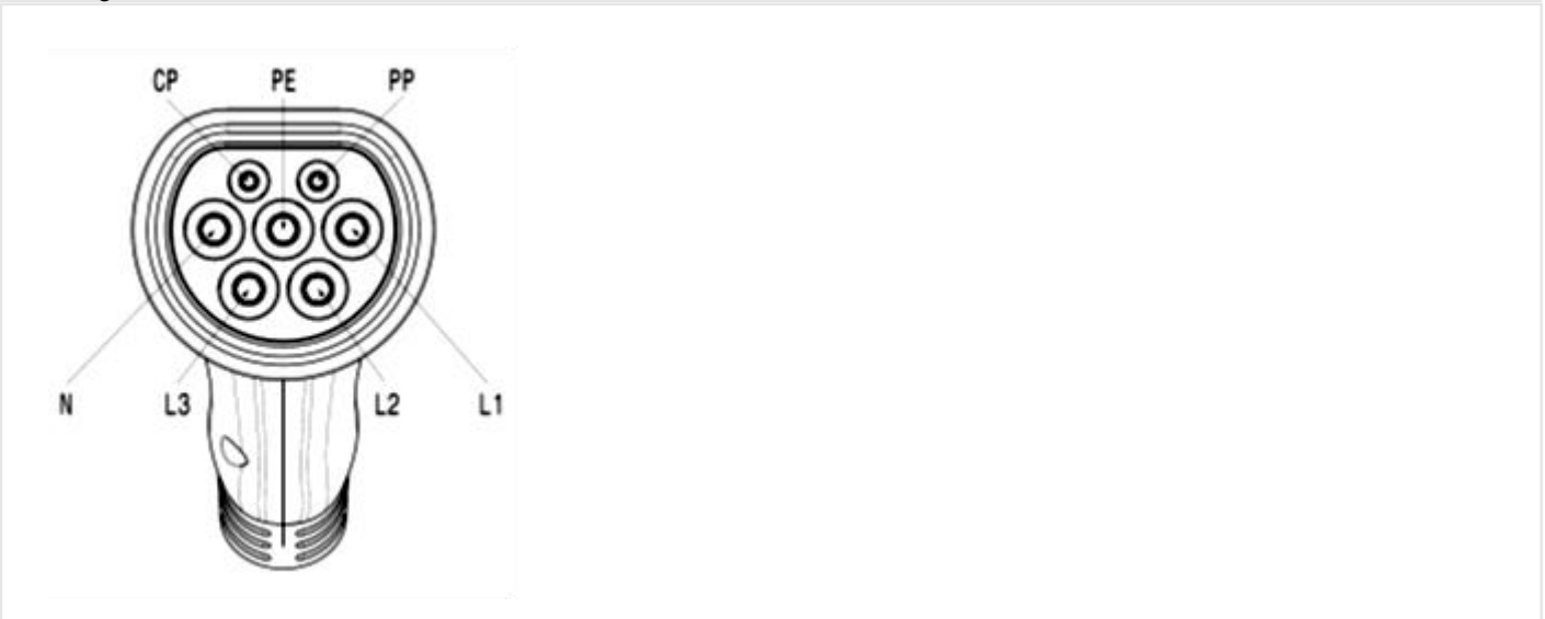
Pin assignment of the female vehicle connector
