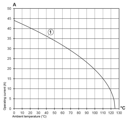
① Conductor cross-section 4 mm² Current rating of the Han E<sup>®</sup> contacts
