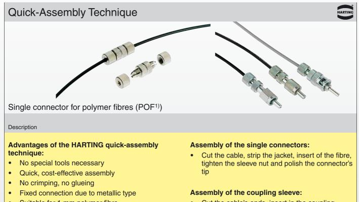
Suitable for 1 mm polymer fibre • (2.2 mm jacket)
