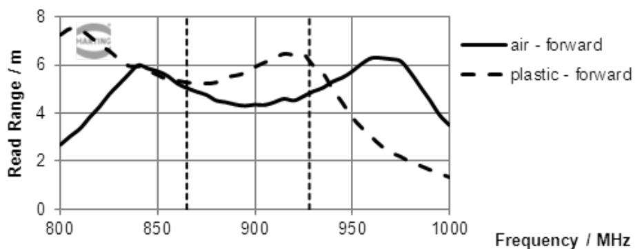
Theoretical Read Range measured in free field conditions (radiated power – 2 W ERP).
