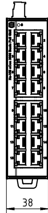
for mounting rail acc. to DIN EN 60715
