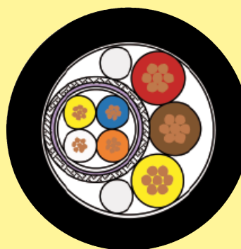
Structure Hybrid cable
