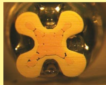
Crimp-cross section HARTING crimp profile
