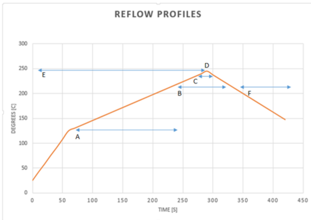
Figure 5-1: Reflow Temperature Profile
