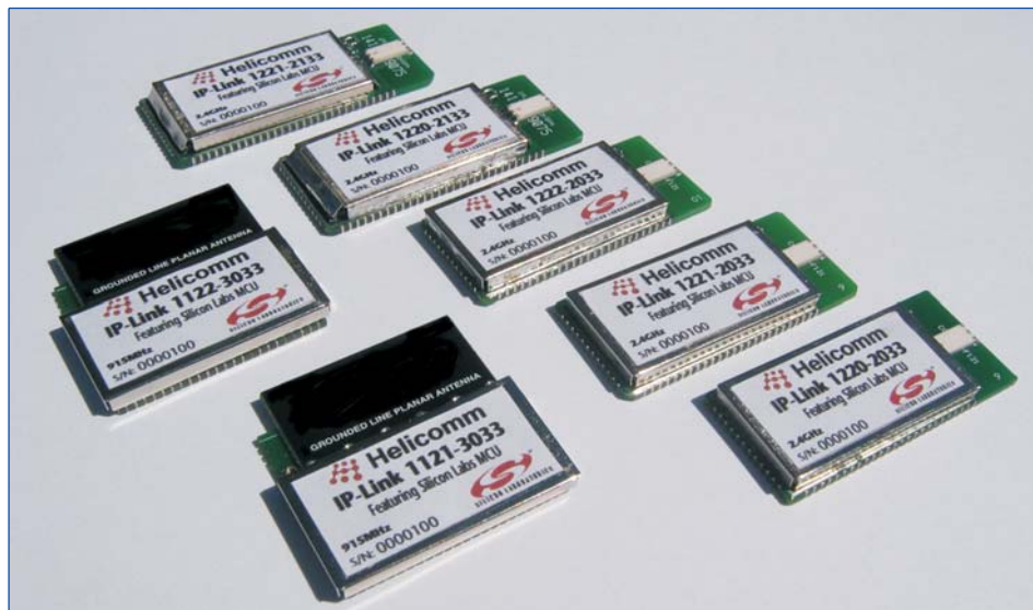
Helicomm's industry leading, 8051-based IP-Link Modules support both ZigBee & IP-Net solutions and 2.4GHz & 915MHz frequencies.
