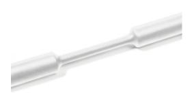
Heat Shrink Tubing, 4' Long Stick, 2:1 Shrink Ratio, 1.25", 31.8/15.4 Dia, PO, White, 10/pkg
