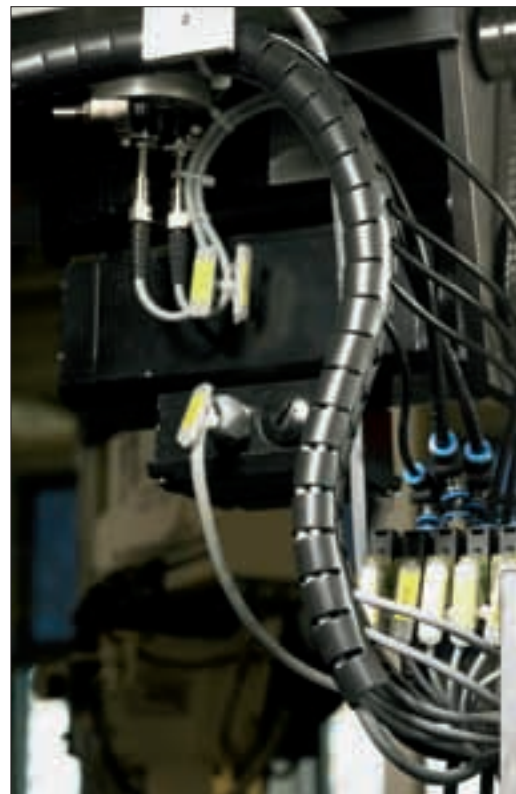
Cables can be branched off at any point for better, more flexible protection.
