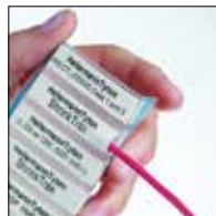
Step 3 Insert wire into marker
