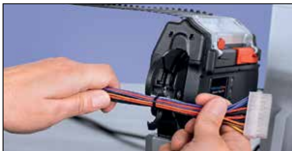
Application with the Bench Mount Kit CPK.
