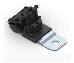
Ratchet P-Clamp, 0.24 - 0.54" Bundle Dia, 180° Short, 0.26" Hole Dia, PA66HIRHSUV/ST/ZN, Black, 5/bag
