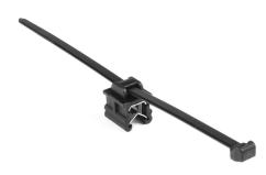
Outside Serrated Cable Tie & Edge Clip, 6.0" Long, EC9, 1-3 mm Panel, 50lb, PA66HS, Black, 500/pkg
