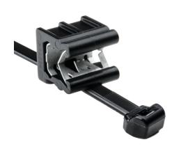
Outside Serrated Cable Tie & Edge Clip, 8.0" Long, EC23, 3 - 6 mm Panel, 50lb, PA66HS, Black, 500/pkg
