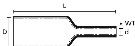
Heat Shrinkable Tubing 4:1 with adhesive.
