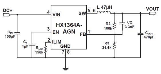
\* The output voltage is set by R2 and R3:  $V_{OUT}$  = 1.20V • [1 + (R2/R3)].
