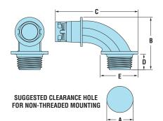
Material Nvlon 6/6 Certifications cPUs Certified to both Canadian and U.S. Requirements File E121095 Flammability Rating 941/-2 Temperature Range -22°F (-30°C) to 221°F (105°C) IP Rating IP 64
