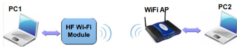
Figure 31. STA Interface Debug Connection
