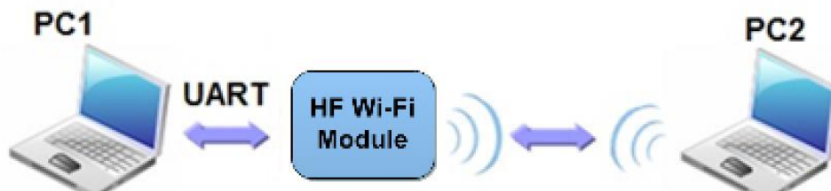
Figure 32. AP Interface Debug Connection
