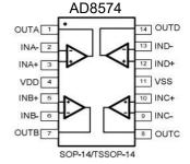
Figure 1. Pin Assignment Diagram
