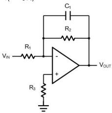
Figure 5. Low Pass Active Filter
