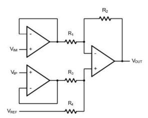
Figure 6. Instrument Amplifier
