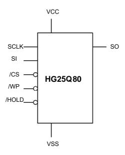
Figure 2. Pin Configuration SOP8L/DIP8L
