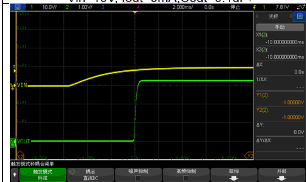
Vin=10V, Iout=30mA, Cout=0.1uF
