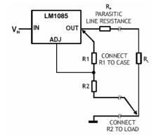
True remote load sensing it is not possible to provide, because the LM1085 is a three terminal device. The resistance of the wire connecting the regulator to the load will limit the load regulation.
