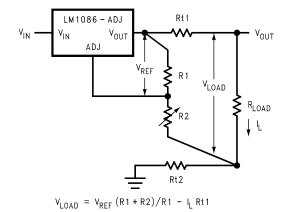
Figure 21. Best Load Regulation using Adjustable Output Regulator
