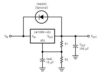
Figure 22. Regulator with Protection Diode
