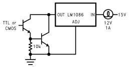
Figure 32. High Current Lamp Driver Protection
