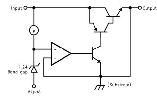
Figure 18. Basic Functional Diagram for the LM1086, excluding Protection circuitry
