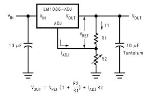
Figure 19. Basic Adjustable Regulator
