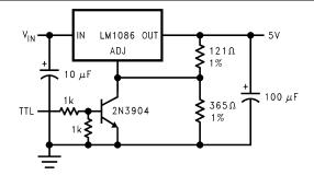
Figure 28. 5V Regulator with Shutdown
