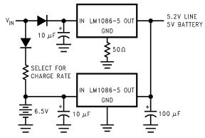
Figure 33. Battery Backup Regulated Supply
