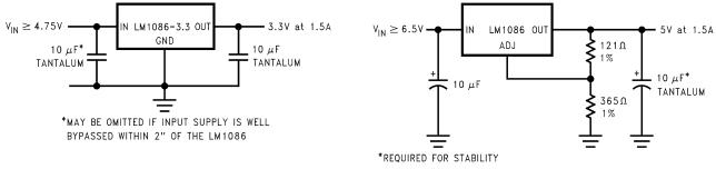
Figure 25. 5V to 3.3V, 1.5A Regulator
