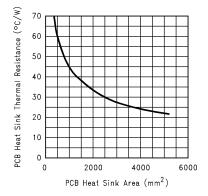
Figure 24. Heat sink thermal Resistance vs. Area
