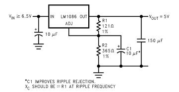
Figure 34. Ripple Rejection Enhancement
