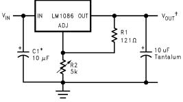
\*NEEDED IF DEVICE IS FAR FROM FILTER CAPACITORS  $V_{OUT} = 1.25V(1 + \frac{R2}{R1})$
