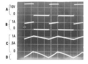
V<sub>OUT</sub> = 5V A: Output Pin Voltage, 10V/div B: Output Pin Current, 1A/div C: Inductor Current, 0.5A/div D: Output Ripple Voltage, 20 mV/div,
