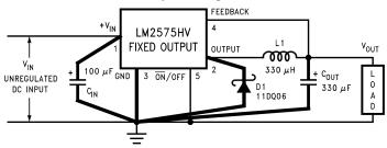
$C_{\text{IN}}$  — 100  $\mu\text{F}$ , 75V, Aluminum Electrolytic
