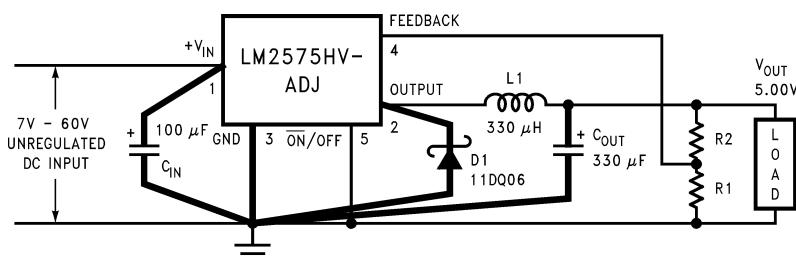
$$V_{OUT} = V_{REF} \left( 1 + \frac{R_2}{R_1} \right)$$
