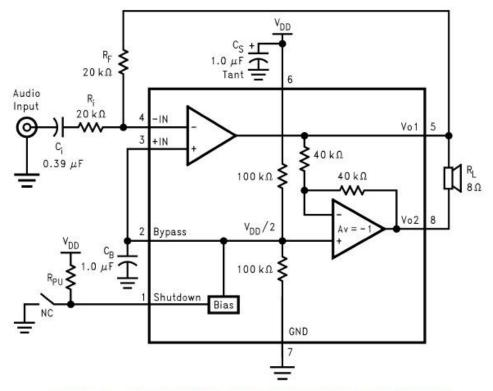
Figure 3. Typical Audio Amplifier Application Circuit
