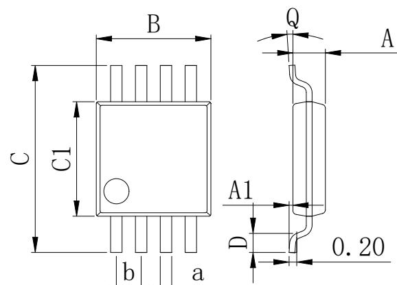
Dimensions In Millimeters(MSOP-8)
