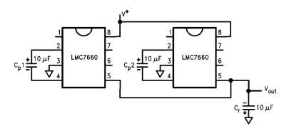
FIGURE 5. Lowering Output Resistance by Paralleling Devices
