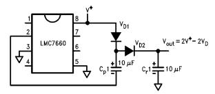
FIGURE 9. Positive Voltage Multiplier
