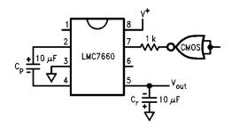
FIGURE 4. Synchronizing to an External Clock
