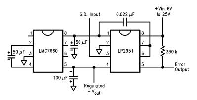
FIGURE 12. Regulated –5V with 200 µA Standby Current
