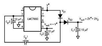
FIGURE 10. Combined Negative Converter and Positive Multiplier
