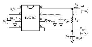
FIGURE 1. LMC7660 Test Circuit
