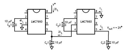
FIGURE 6. Higher Voltage by Cascade
