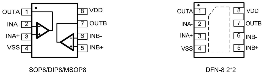
Figure 1. LMV602 Pin Assignment Diagram
