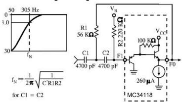
As a high pass filter, with the components shown in Figure 6 the filter will keep out 60 Hz (and 120 Hz) hum which can be picked up by the external telephone lines.
