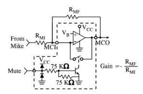
The muting function (Pin 12), when activated, will reduce the gain of the amplifier to = -39 dB (will RMI = 5.1 K $\Omega$ ) by shorting the output to the inverting input (see Figure 5). The mute input has a threshold of 1.5 volt, and the voltage at this pin must be kept withing the range of ground and VCC. If the mute function is not used, the pin should be grounded.
