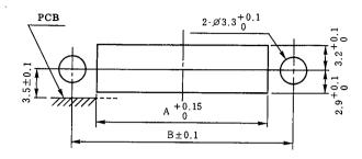
Unit: mm No. of HRS No. Part No. CL231-3006-8 6 18.06 3110- 6S 23.96 CL231-3001-4 3110- 8S 20.6 CL231-3008-3 3110-12S 25.68 31.58 CL231-0018-0 3110-16S 30.76 36.66 CL231-0021-5 3110-14SB 28.22
