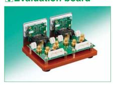
Evaluation boards are available to check the operating characteristic of the plug harness.
