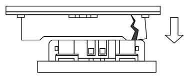
② It could apply excessive mechanical stress to single side of the contact.
