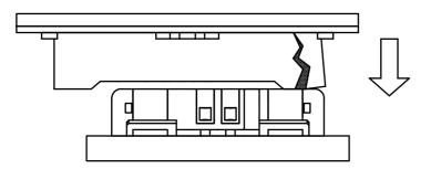
② It could apply excessive mechanical stress to single side of the contact.
