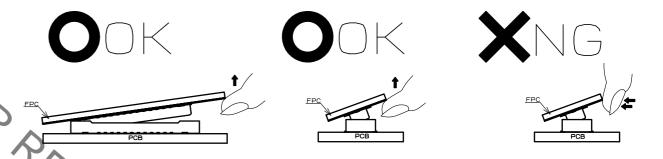
FPC IS NOT RIGID. THE CONNECTOR CAN BE BROKEN. PLEASE CHECK THE ACTION OF THE FPC TO BE USED REPEATEDLY AT THE TIME OF TRIAL PRODUCTION. BE CAREFUL TO UN-MATE THEM FROM THE PITCH DIRECTION. DM THE CORNER CAN ALSO RISK TO PUTTING STRESS ON CONTACTS.
