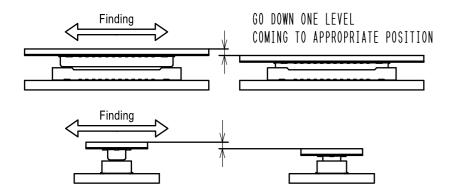
(2) WHEN GUIDING. THE CONNECTORS ARE ALIGNED PARALLEL TO EACH OTHER, WITH LONGITUDINAL AND LATERAL MOVEMENTS RESTRICTED. MATE THEM PROPERLY BY APPLYING FORCE IN THIS CONDITION.
