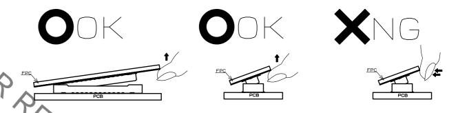
(3) IF THE EPC IS NOT RIGID, THE CONNECTOR CAN BE BROKEN. PLEASE CHECK THE ACTION OF THE FPC TO BE USED REPEATEDLY AT THE TIME OF TRIAL PRODUCTION. BE CAREFUL TO UN-MATE THEM FROM THE PITCH DIRECTION, PULLING IT FROM THE CORNER CAN ALSO RISK TO PUTTING STRESS ON CONTACTS.
