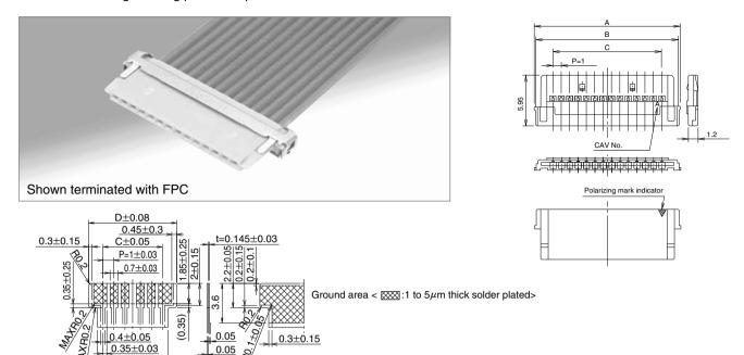
Signal area < 8883:1 to  $5\mu$ m thick solder plated>
