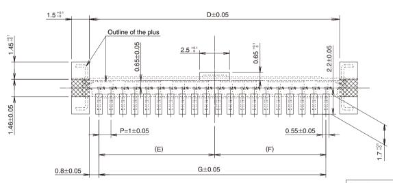
Conductive traces in this area must be covered by dielectric compound.
