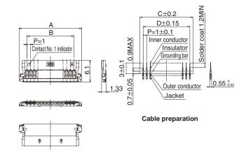
Note 1: Connectors are designed to allow termination without cutting of the pitch loss prevention tape.
