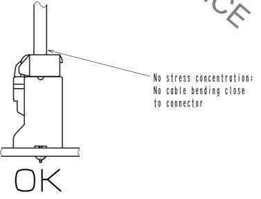
2) Since this product uses thick wires, a larger load is applied to the connector when inserting/extracting or routing the wires. Please use a retainer to reduce the load on the connector.
