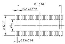
Recommended solder paste thickness: 120  $\mu$ m
