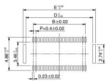
Recommended solder paste thickness: 120  $\mu$ m
