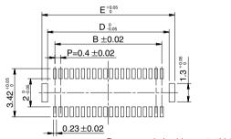
Recommended solder paste thickness: 120  $\mu$ m
