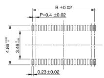
Recommended solder paste thickness: 120  $\mu$ m
